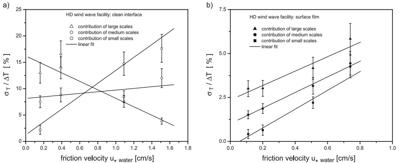
**Figure 2.** Contribution of small-, medium-, and large-scale turbulence to the temperature gradient across the thermal sublayer. The standard deviation of a certain scale (level 0, 2, and 4 of the Laplacian pyramid) of the temperature distribution is divided by the estimated skin-bulk temperature difference and plotted versus friction velocity (a) for a clean interface and (b) while a surfactant (Triton X-100, bulk concentration 3 ppm) was present.
