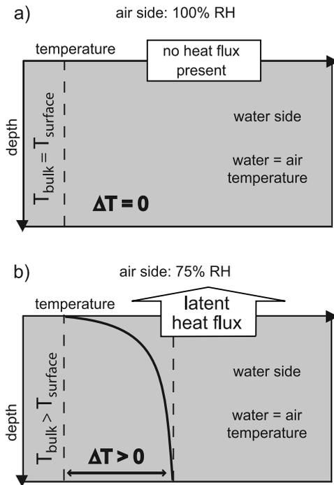
**Figure 3.** The two operating modes of the wind-wave facility: (a) water and air have the same temperature, relative humidity is  $\approx 100\%$ , no latent, sensible, or net radiative heat flux at the water surface is present. (b) Flushing the air space with dry air ( $RH \approx 75\%$ ) creates an evaporative heat flux density that forces a skin-bulk temperature difference  $\mathcal{O}(0.1 \text{ K})$  across the thermal sublayer  $\mathcal{O}(100 \mu\text{m} - 1 \text{ mm})$ .
