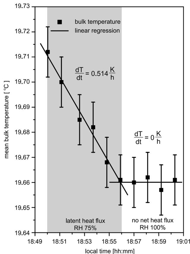
**Figure 6.** Mean temperature of the water bulk in the wind-wave facility during one period of heat flux switching.
