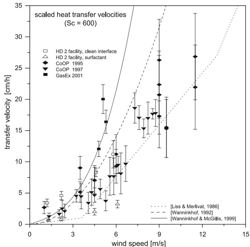
**Figure 8.** Scaled transfer velocities ( $k_{600}$ ) during the CoOP 1995 (data adapted from *Haussecker* [1996]), CoOP 1997, and GasEx 2001 experiments and in the Heidelberg wind-wave facility plotted versus wind speed. For comparison the empirical relationships of *Liss and Merlivat* [1986], *Wanninkhof* [1992], and *Wanninkhof and McGillis* [1999] are shown.
