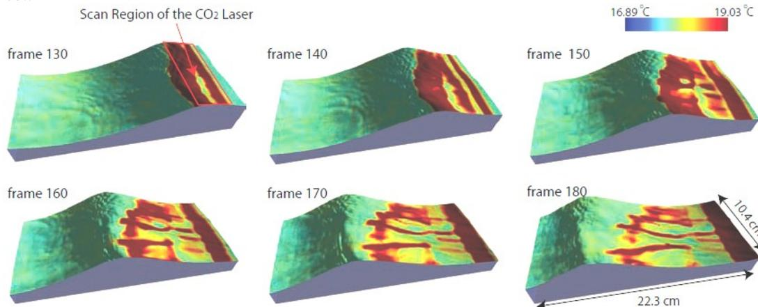
**Figure 2: Combined visualization of surface temperature and waves. For a wind speed of 6 m/s elongated streaks appear which can be attributed to micro Langmuir circulation (Melville et al. (1998)). The initial temperature signature is artificially generated by a CO<sub>2</sub>-Laser and observed by an infrared camera. Wind is blowing from the right to the left. (The time interval between two consecutive snapshots (which are 10 frames apart) is 0.032 seconds).**
