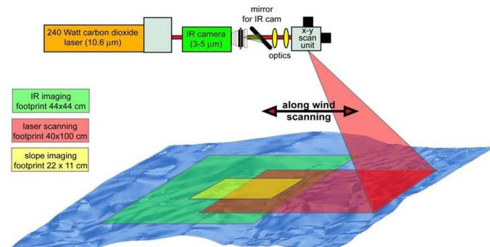
**Figure 1: Schematic drawing of the overlapping footprints of the CISG camera (yellow) and the infrared camera (green), as well as the scanning range of the infrared laser (red).**
