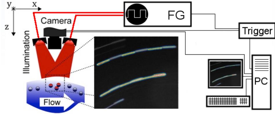
Figure 1: Experimental set-up for the automated measurement of 3D3C flow-fields in the air-water boundary layer. The intensity variation along the streaks enables an extraction of the particle depth.
