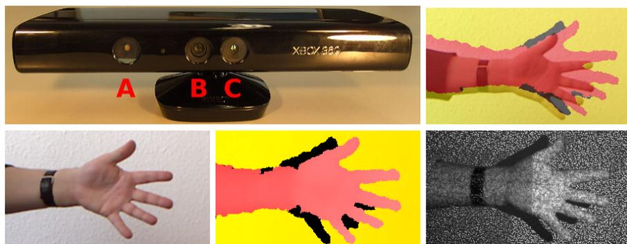
**Fig. 1.** *Kinect* device and its raw data output. **Top:** *Kinect* device with projector (A), color cam (B) and IR cam (C); color and depth channel overlayed. **Bottom** (left to right): raw color image; pseudo-color coding of the 11bit depth image provided by the on chip depth estimation; raw IR image showing the projected point pattern.
