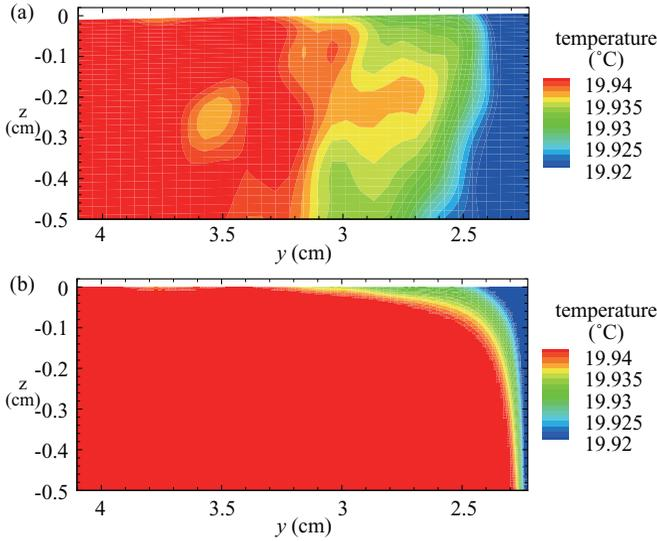
**Figure 4** Temperature field for one-half of eddy. (a) detected from simulation result. (b) predicted by eddy-renewal model. The left boundary in this one-half of eddy is corresponded to the location of upwelling, and the right boundary is corresponded to the location of downwelling.
