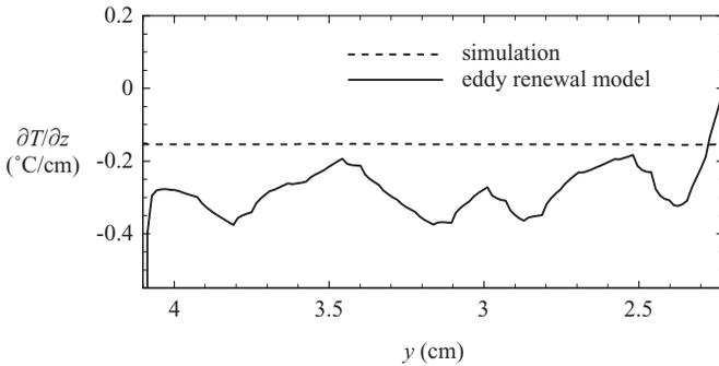
**Figure 5** Spatial variation in vertical gradient of surface temperature on a one-half of eddy. Solid line: estimated by eddy-renewal model; dash line: simulation result.
