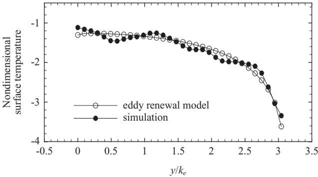
**Figure 2** Fitting the surface temperature of a one-half of eddy detected from simulation result with the solution of eddy-renewal model.  $k_e$  is the wavenumber of the eddy.
