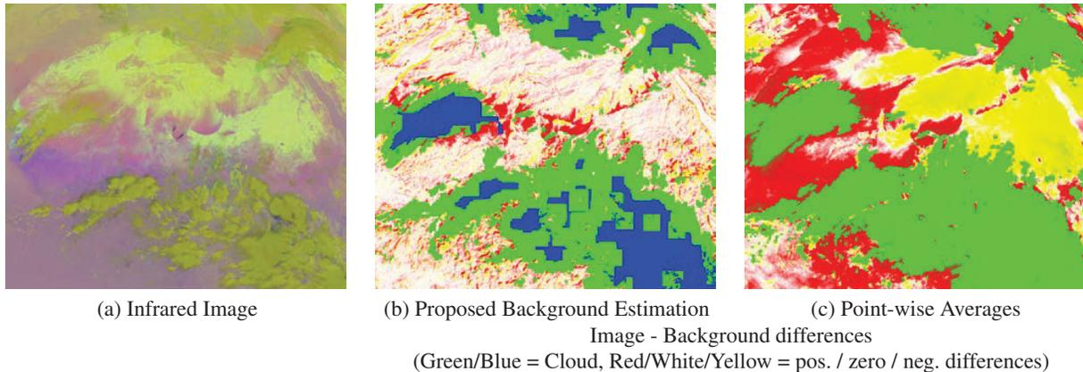
**Fig. 1.** Given a sequence of infrared images (a), a background can be estimated. If the background is estimated, as proposed, from non-cloud, non-dust pixels then the image-background difference (b) reveals the presence of dust clouds (red), but if point-wise averages are used to find the background, then the image-background difference (c) has significant contamination.
