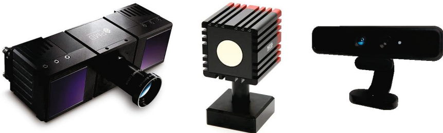
Fig. 1. Different ToF phase based camera models available in the market. A PMD CamCube 2.0 (left), a swissranger SR 400 (middle) and a DepthSense DS325 (right).
